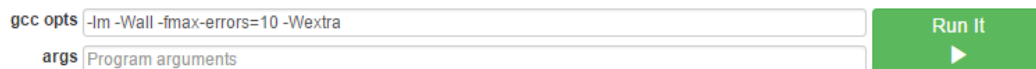
Figure 2.10: Controls for compiling and running the program, setting options for gcc, and specifying the command-line arguments passed to the program
